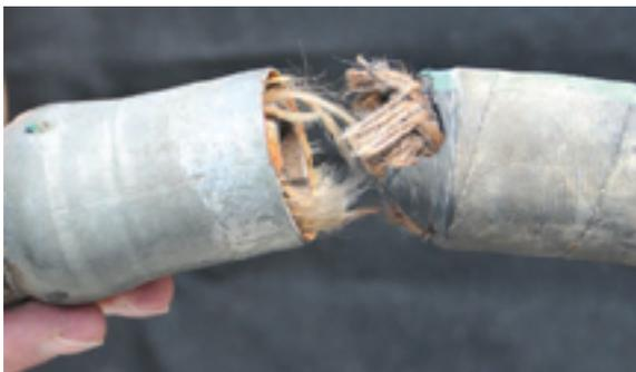
**Failure due to Kinking at Fitting**
